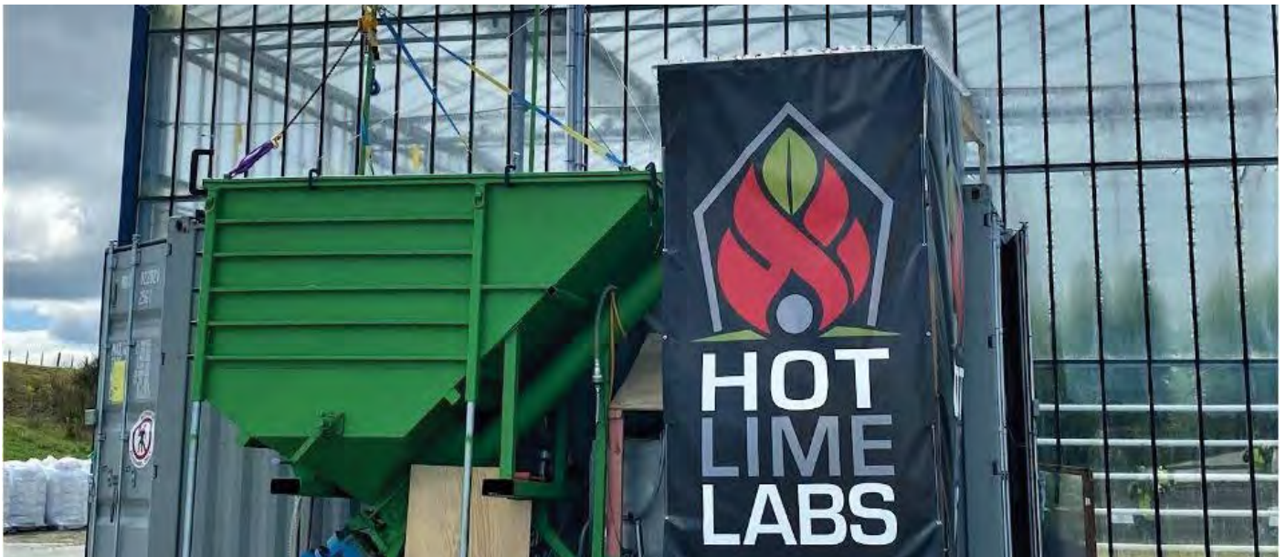
Hot Lime Labs pilot system, producing CO 2 from waste wood
