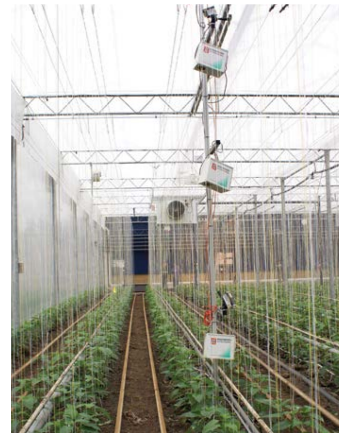
PE requires some extra measurements: at least an extra box for temperature and humidity above the screen, and a plant temperature sensor
