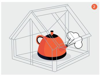
A third form of heat is latent heat, which means hidden heat or hidden energy. Latent heat cannot be felt, unlike radiative heat and convective heat. Latent heat is the presence of water vapour in the air. Note that water vapour is invisible, unlike fog or mist that consists of small visible water droplets.
