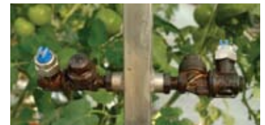
Fig. 2. 80° flat fan nozzles facing upwards at a 45° angle.
