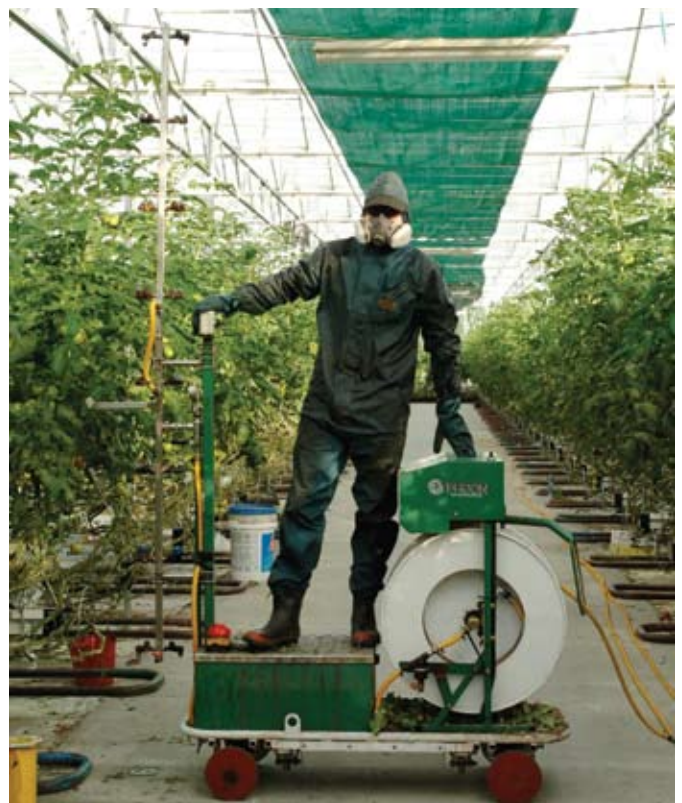
Fig. 3. Vertical pipe-rail boom sprayer. When travelling down rows the spray boom follows the person, thereby minimising worker contact with chemicals.
